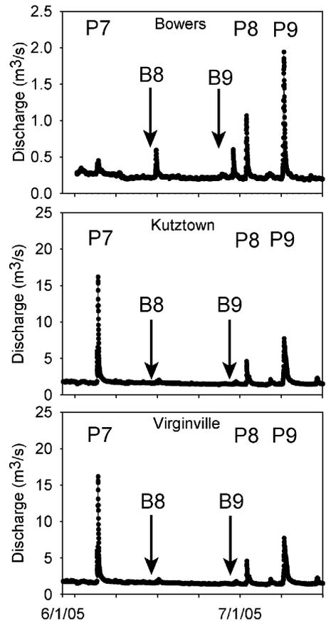
Figure 2. Gauge data from three stations in Sacony Creek watershed from December 2004 to January 2005. These data illustrate how discharge data are compiled moving downstream for both peak and base flow events. Discharge labels correspond with either peak flows (e.g., P7, P8, P9) or base flows (Table 3).
