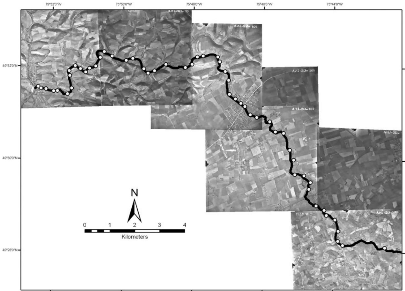
FIGURE 4. The Location of the Width Measurements (circles) on Sacony Creek. The background image is from 1946, and the river itself has been darkened for identification.
