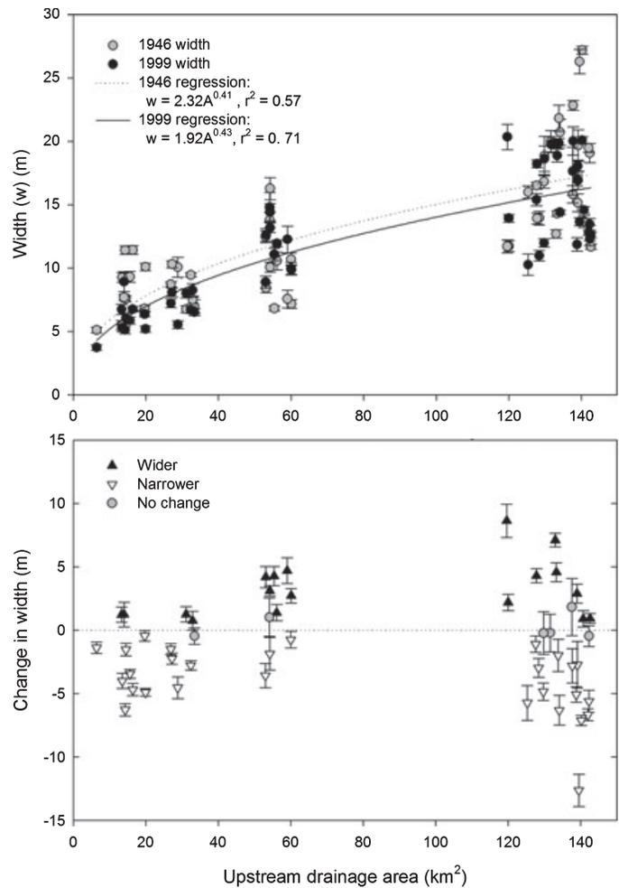
FIGURE 6. The Measured Widths (top) for Sacony Creek From 1946 (gray circles) and 1999 (black circles), and the Change in Widths (bottom) Over That Time. The widths did not systematically change in Sacony Creek. The gaps in measured widths are from tributaries increasing the upstream drainage area, not from large distances between width measurements (Figure 4).
