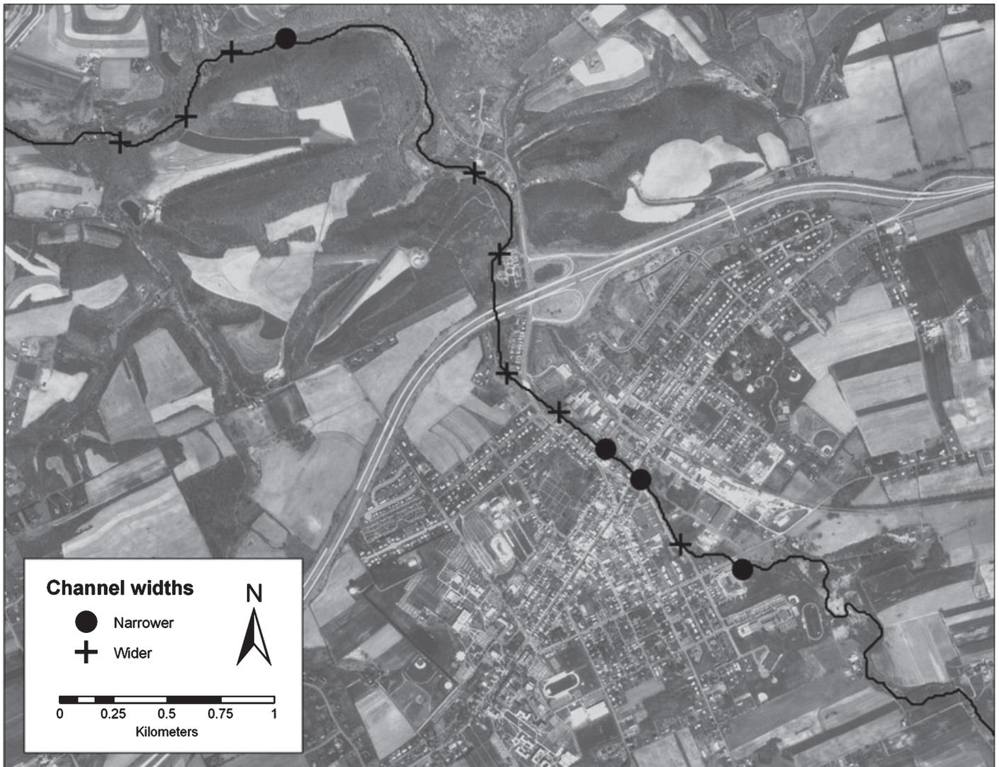
FIGURE 11. The Town of Kutztown, Pennsylvania (the gridded pattern in the central portion of the photograph), and Sacony Creek With Its Measured Widths. The widths that increased (+) from 1946 to 1999 are concentrated downstream of Kutztown, while those that narrowed (●) are distributed along the entire river. The widened channels extend for 3.8 km downstream of Kutztown, and suggest a downstream limit to the effects of Kutztown's increased urban area.
