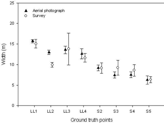
FIGURE 7. The Comparison of Survey Measurements of the Channel Width Along a Reach to the Widths Measured From Aerial Photographs. The x-axis labels refer to the survey positions listed in Figure 1 for Little Lehigh Creek (LL) and Sacony Creek (S).
