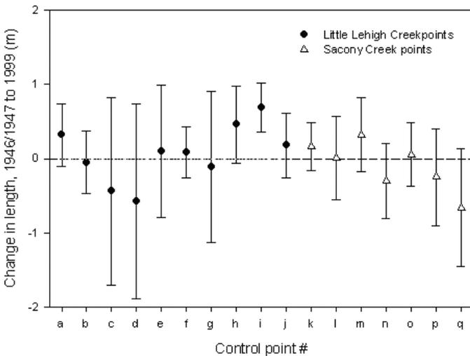
FIGURE 8. The Comparison of Measured Ground Controlled Points From the 1947 and 1999 Georeferenced Aerial Photographs From the Two Watersheds. The measurements do not systematically change between the two sets of photographs, implying that there are not spatial differences due to georeferencing errors.
