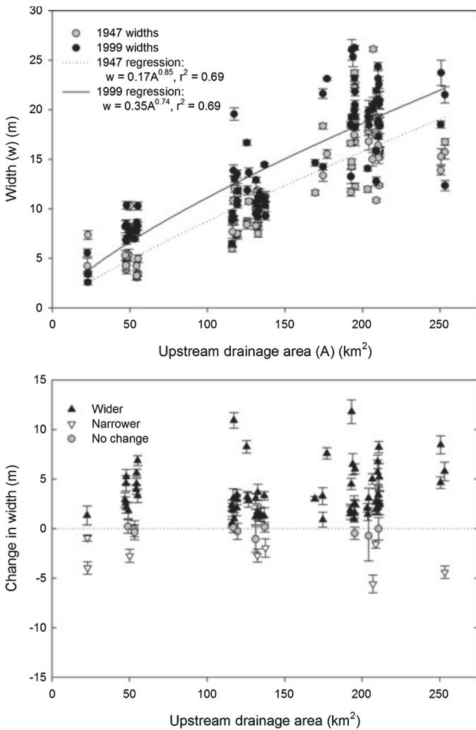
FIGURE 5. The Measured Widths (top) of the Little Lehigh Creek From 1947 (gray circles) and 1999 (black circles), and the Change in Widths (bottom) Over That Time. The widths increased on 67 of the 85 measured sites. The gaps in measured widths are from tributaries increasing the upstream drainage area, not from large distances between width measurements (Figure 3).
